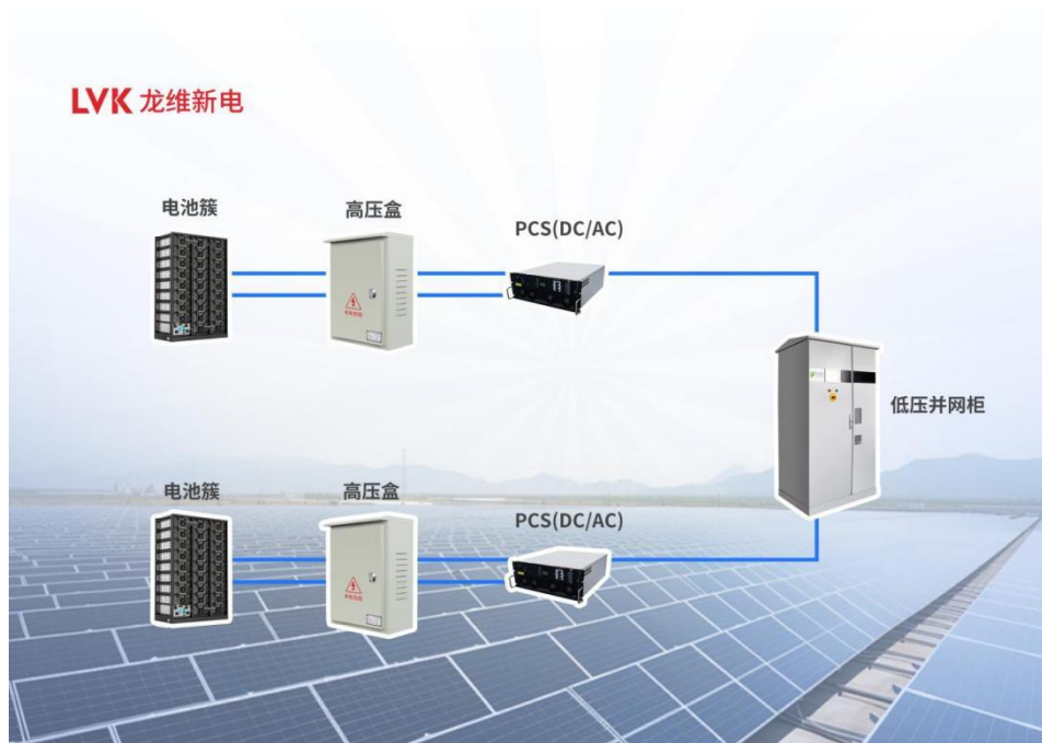
Figure 1-2: 522kWh Energy Storage Outdoor Cabinet Parallel Topology (battery-PCS-Grid-Connected Cabinet)
