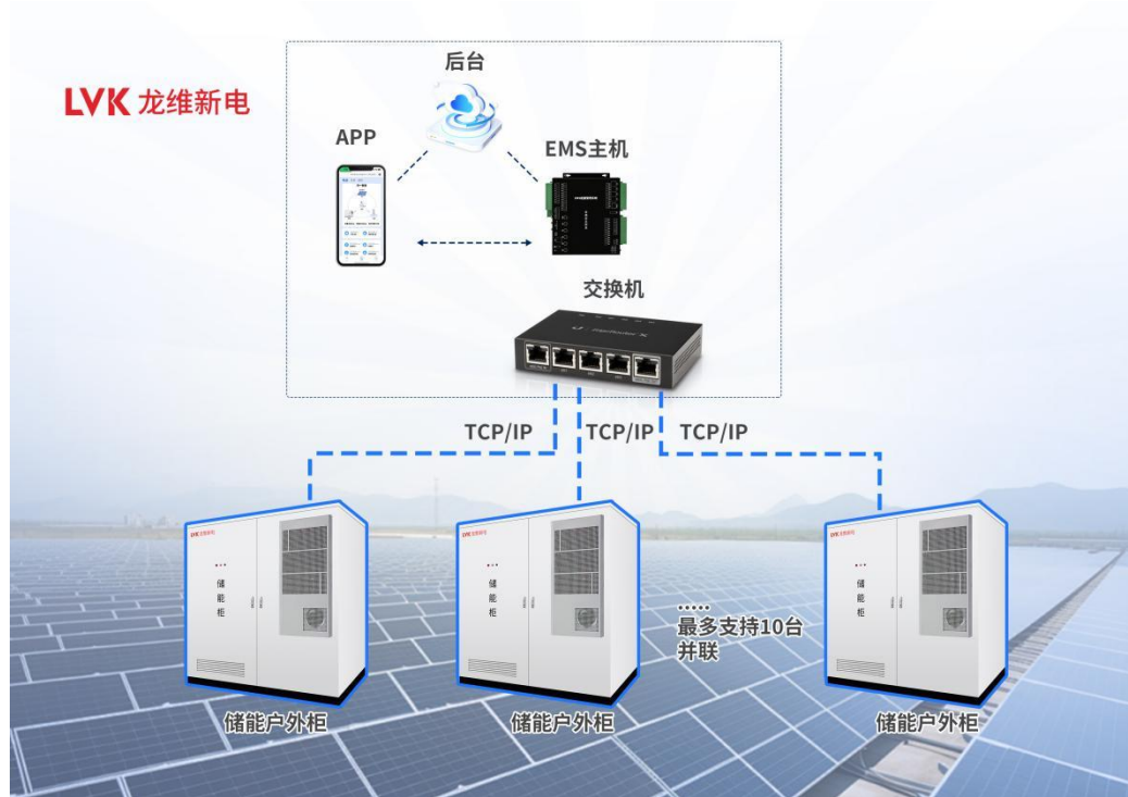
Figure 2-4 EMS Communication Architecture Diagram
